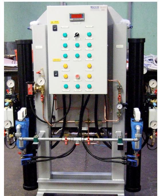
All Silicair Dryers models are CE marked as standard and are custom selected to meet your specific requirements based on the exact operating parameters for your process. To obtain the correct model to meet your requirements please contact us with your inlet flow, pressure, temperature and required outlet dewpoint to meet the nominated medical air standard and specification.
